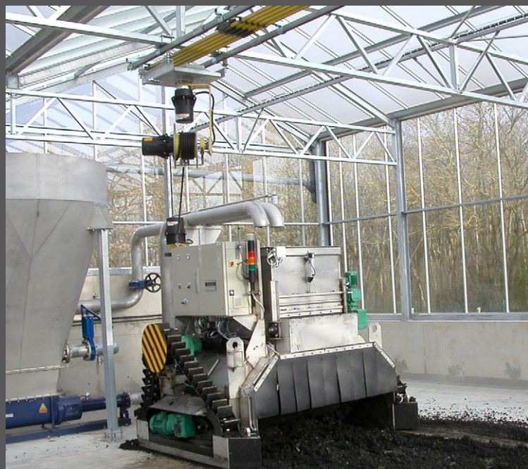
Customized solution with conductor rail, spring reel and slip ring assembly for sludge drying systems
